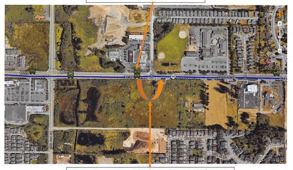
Relocate and improve existing east bound bus stop (ID #3129) at  $132^{nd}$  St SE and  $39^{th}$  Ave SE to the right turn pocket being developed with the new traffic signal, east of  $39^{th}$  Ave SE. Improvements include Type 4 bus pad and shelter.
