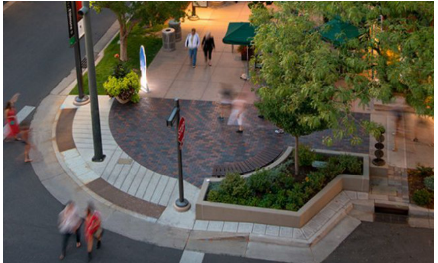
Figure 95 - Curb Bulbs with Planting and Seating Elements
